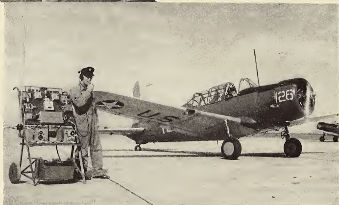
The picture above shows how Waco Flying School's portable control tower can be operated at auxiliary landing areas. It generates its own power, thus eliminating outside attachments, and can be transported by jeep.
